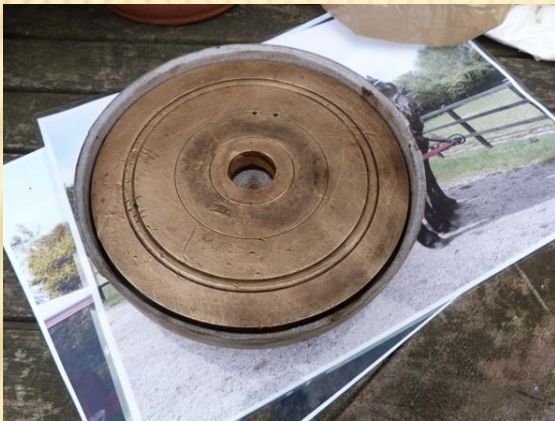
New leather cup washers for the split pistons.
