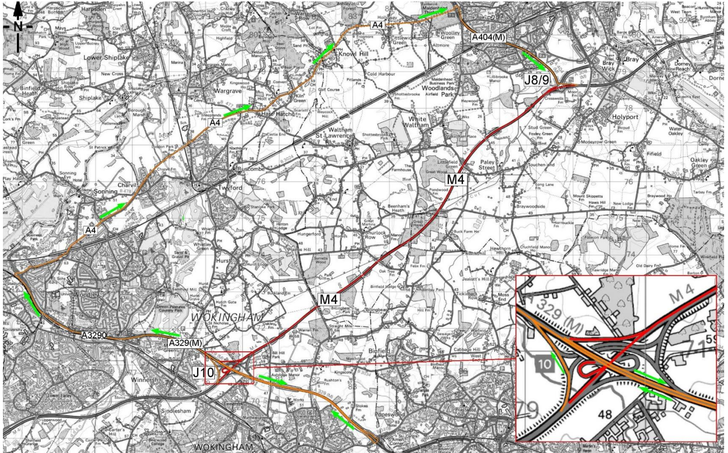
Route for eastbound traffic during night time closures. NB: westbound traffic will use the reversed route.
